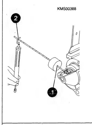
Checking armature braking torque
